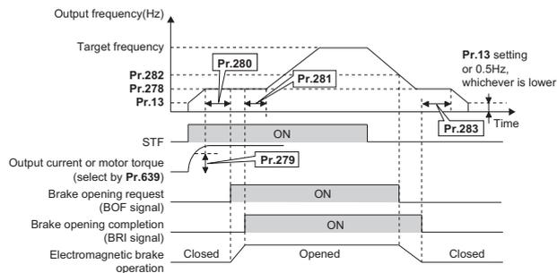
When **Pr.292 = "8"** (without brake opening completion signal input)
