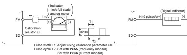
\*1 Not needed when the operation panel (FR-DU08) or parameter unit (FR-PU07) is used for calibration. Use a calibration resistor when the indicator (frequency meter) needs to be calibrated by a neighboring device because the indicator is located far from the inverter. However, the frequency meter needle may not deflect to full-scale if the calibration resistor is connected. In this case, calibrate additionally with the operation panel or parameter unit.
