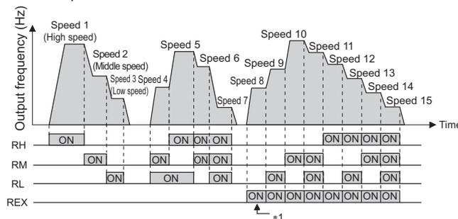
\*1 Operates at the frequency set in **Pr.6** when RH, RM, or RL is OFF and REX is ON while **Pr.232 Multi-speed setting (speed 8)** = "9999".
