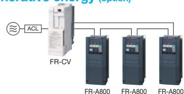
Regenerative power is used at other inverters, and surplus energy is returned to the power supply, resulting in energy saving. The 315K or higher models are inverter-converter separated types, which are suitable for power regeneration. **NEW**
