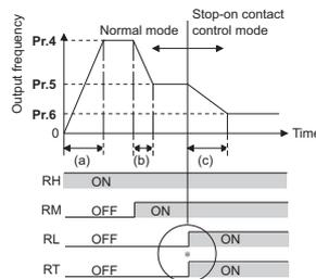
\* Goes into stop-on-contact control mode when both RL and RT switch on. RL and RT may be switched on in any order with any time difference
