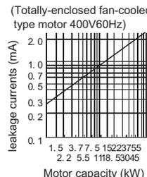
For  $\Delta$  connection, the amount of leakage current is approx. 1/3 of the above value.
