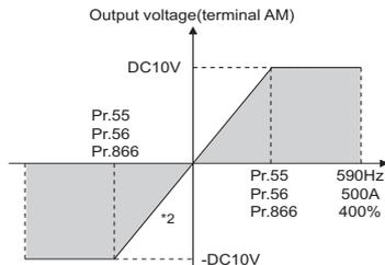
\*2 Minus-sign output is enabled when Pr.290 Monitor negative output selection = "1 and 3".
