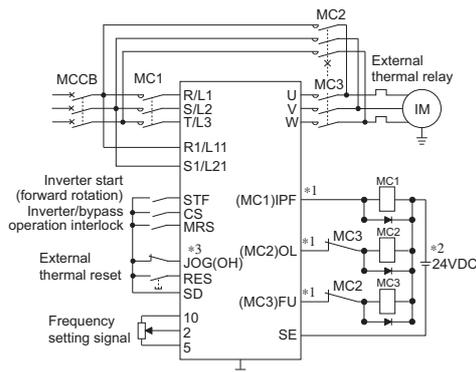
Electronic bypass sequence connection diagram
