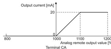
When **Pr.158 AM terminal function selection** = "87, 88, 89, or 90", an analog voltage can be output from the terminal AM.
