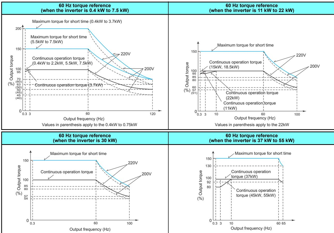
The maximum short-time torque indicates the maximum torque characteristics within 60 s. For the motor constant under Real sensorless vector control, please contact your sales representative.
