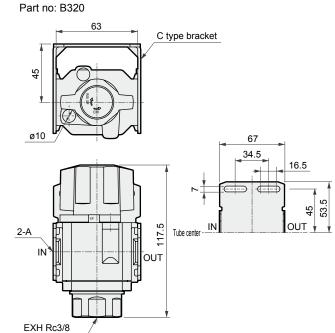
The C type bracket is attached at shipment. C type bracket and piping adapter set can not be used together.
