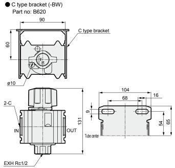
The C type bracket is attached at shipment. C type bracket and piping adapter set can not be used together.
